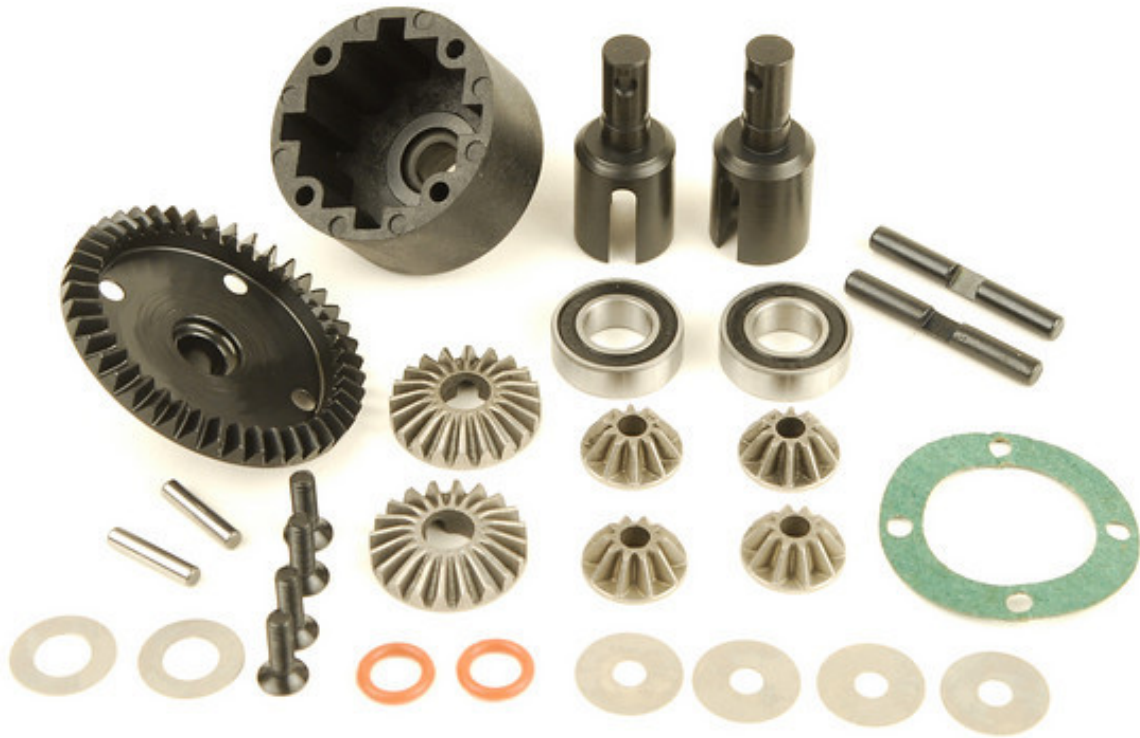
A basic differential. Gears shims and pins. Pretty simple.
